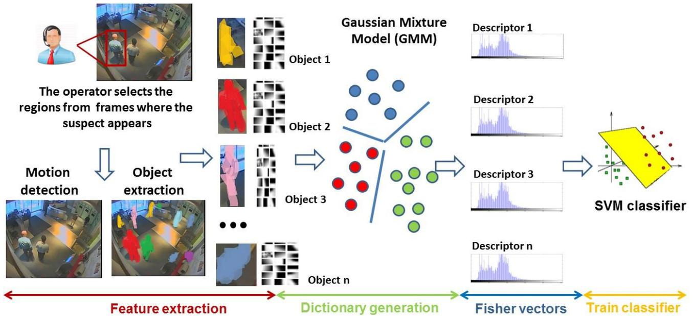
Figure 1. The proposed automated surveillance system: (1) motion detection and feature extraction, (2) dictionary representation, (3) Fisher Kernel representation, (4) SVM classification.
